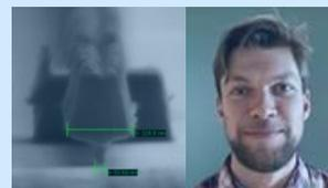
The lift-off has shown to be smoother compared with the previous two-layer resist process and therefore has improved the repeatability.
