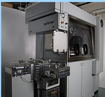
**New hot-wall MOCVD reactor:** Gandalf has been installed at LiU. Tests on flowing heat and active gases have been successfully performed. *Kevin Olsson*, an industrial Master student, works together with Epiluvac, SweGaN and LiU on optimizing gas flow profile.
