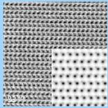
**N-polar GaN/AlN heterostructures:** LiU has successfully developed N-polar GaN on AlN on 4° off-cut SiC (000-1). Current research efforts include optimizing the interface in order to obtain 2DEG with high density and mobility parameters.
